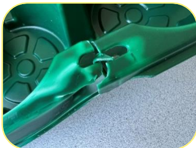
Broken edges, which can lead to injuries, qualify for replacement.
