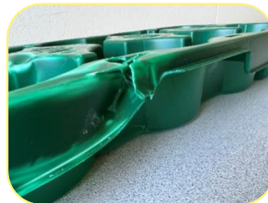
Broken edges, which can lead to injuries, qualify for replacement.
